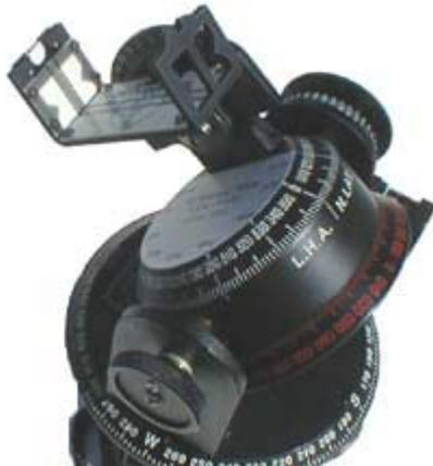
**Figure 7:** Shadow alignment on the rear plate when the Astro-compass is correctly calibrated
