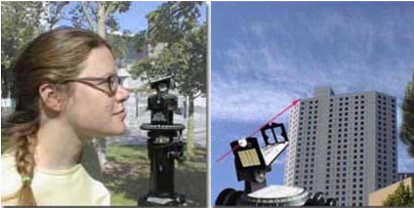
*Figure 10: Sighting altitude, or angular height, with the Astro-compass*
