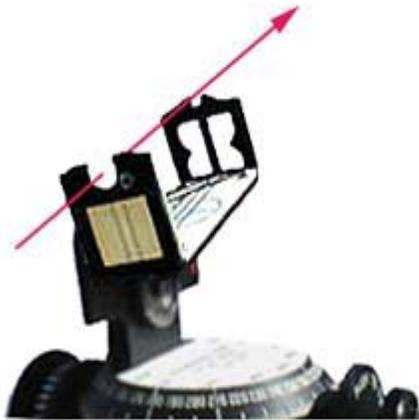
The lens of the rear plate focuses one's eye on the cross hairs so this split view does not cause eye strain. In this example, one is sighting on the location that the sun would be on that day of the year. Be careful not to look directly at the sun when its actual location corresponds to the projected location.
